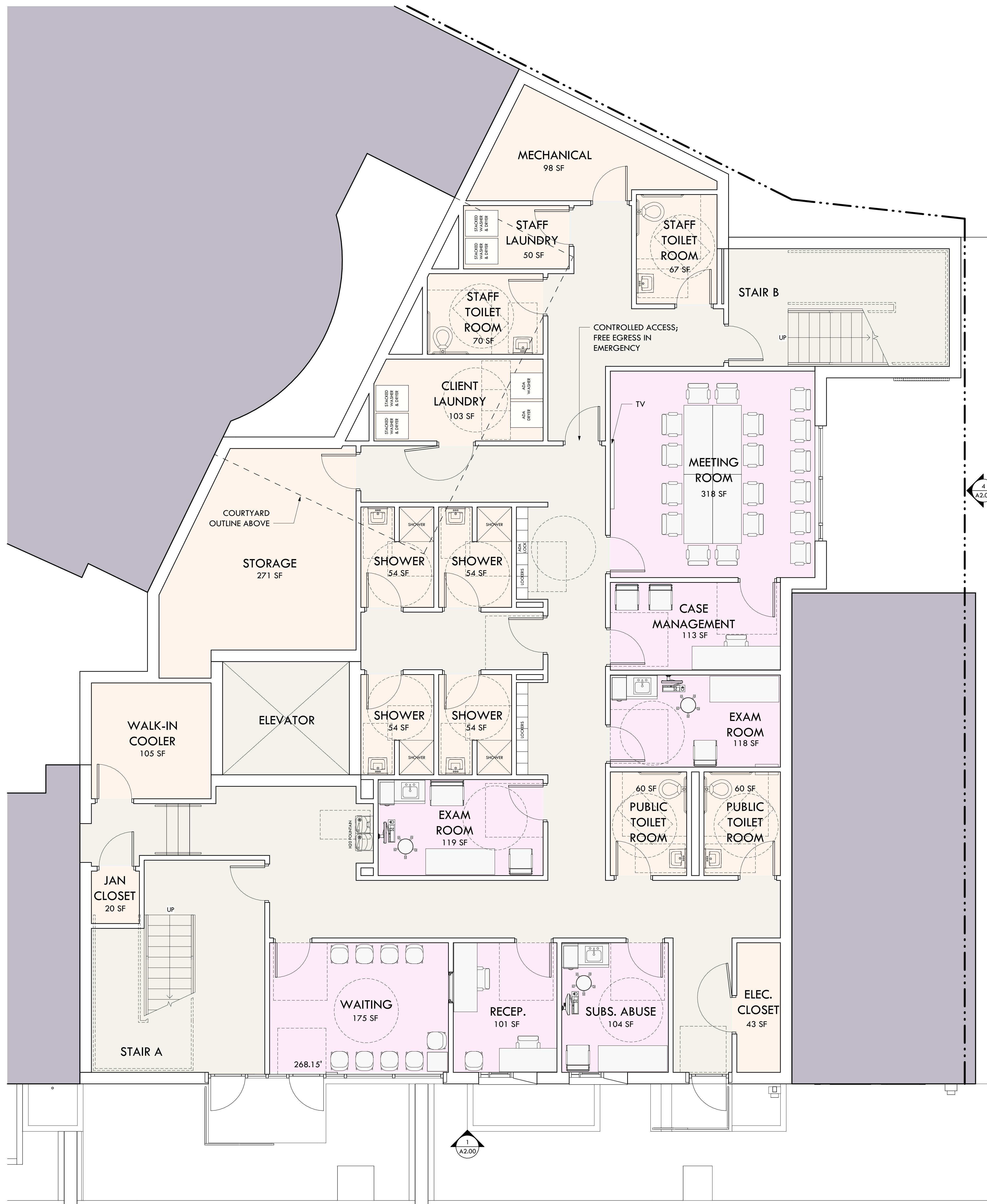
1 ANNEX FIRST FLOOR - PROPOSED PLAN SCALE: 1/4" = 1'-0"
