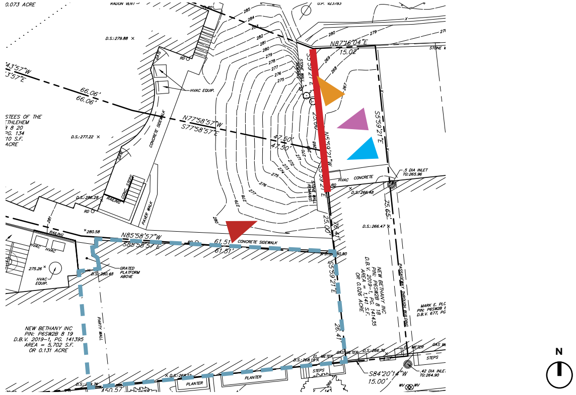
Image 18: Enlarged View of Site Survey Plan, 335-339 West Fourth Street; Survey by Barry Isett Associates, Inc. [For full-size plan, refer to separate drawing package] Blue Outline: Existing Annex; Red Line: Location of collapsed stone retaining wall. Blue Triangle: Image 19, below left; Orange Triangle: Image 20, below right; Magenta Triangle: Image 21, top image next page; Red Triangle: Image 22, bottom image next page.
